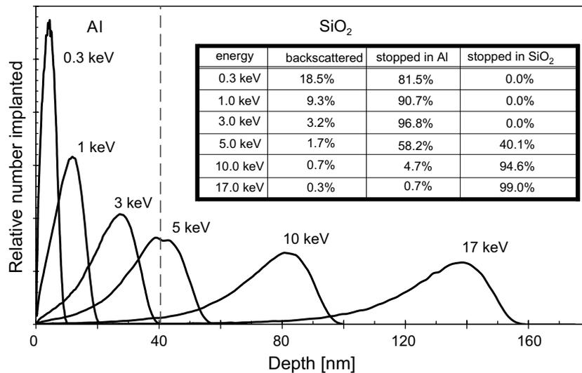
Fig. 10. The implantation profiles for LE- $\mu^+$  in 40 nm thick Al layer on SiO<sub>2</sub> substrate calculated for different implantation energies using TRIM.SP code. Calculation assumes narrow Gaussian energy distribution of the incident muons with a standard deviation of  $\sigma_E = 14$  eV and the incidence angle being perpendicular to the sample surface with  $\sigma_\alpha = 5^\circ$ .
