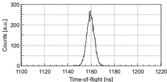
Fig. 8. Time-of-flight histogram of the 9.0 keV LE- $\mu^+$  detected by microchannel plate detector at the sample position. Time zero corresponds to muonium ionization by the laser pulses. Gaussian fit to this histogram yields FWHM pulse duration of 7.5 ns.
