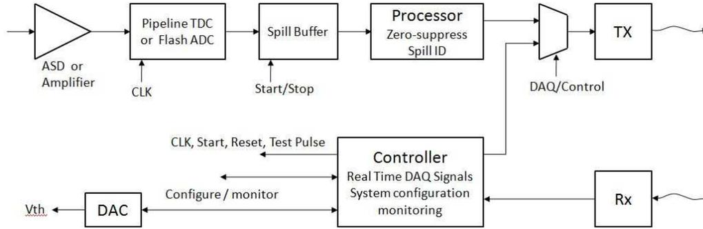
FIG. 68: Block diagram of the front-end board.
