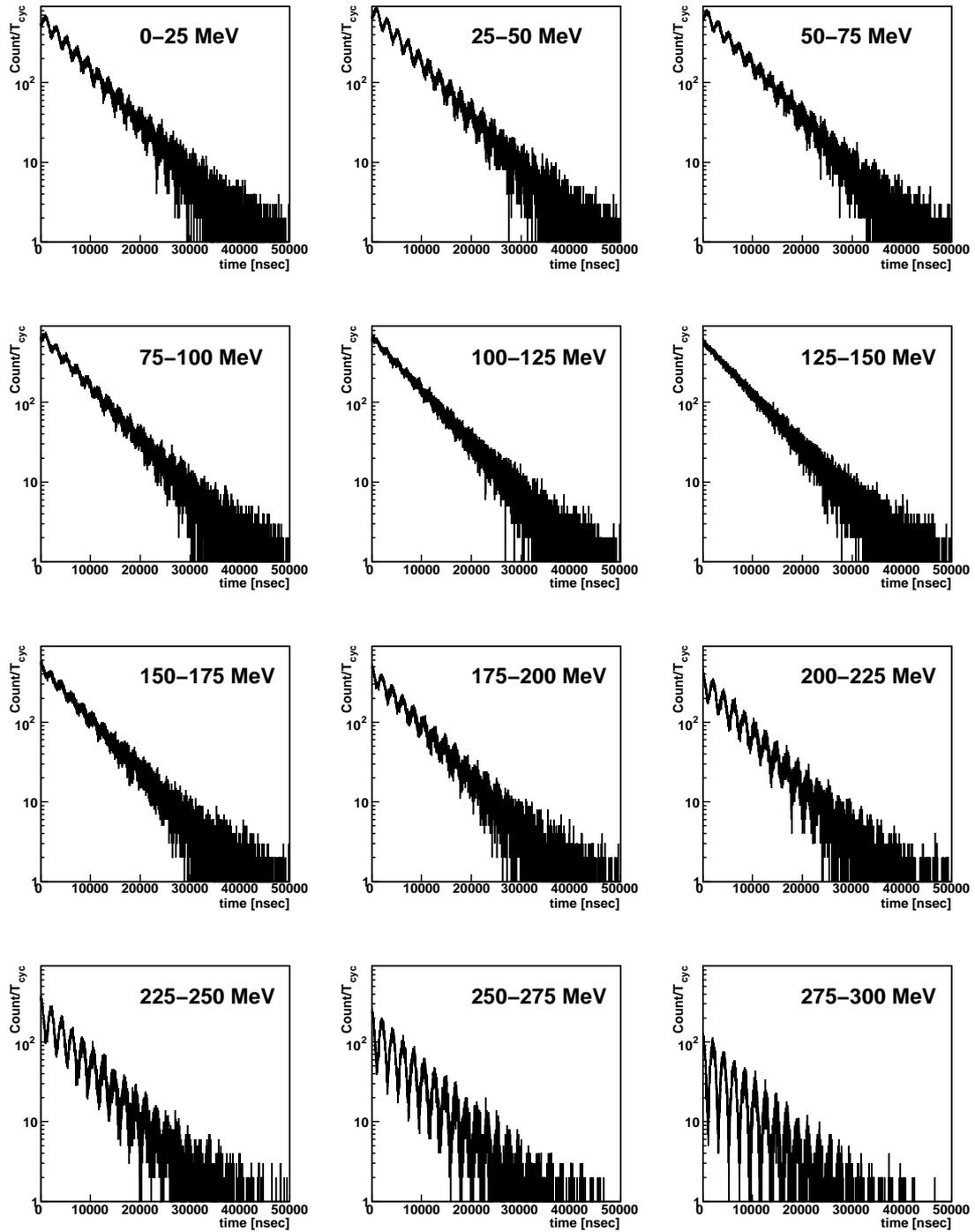
FIG. 60: Positron time spectra generated by GEANT4 for 65M events for several energies, with  $P_{mu} = 1$ . Spectra of  $E_{lab} < 100$  MeV ( $E_{lab} > 175$  MeV) correspond to *backward-decay* (*forward-decay*) in the muon rest frame.
