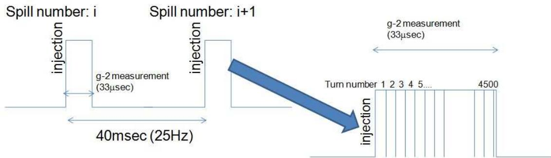
FIG. 65: Time sequence of the  $g - 2$  precession measurement
