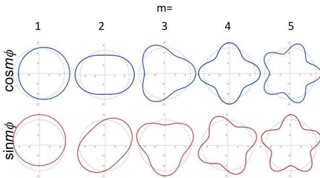
FIG. 48: The structural errors expressed by radial or longitudinal deformation modes.
