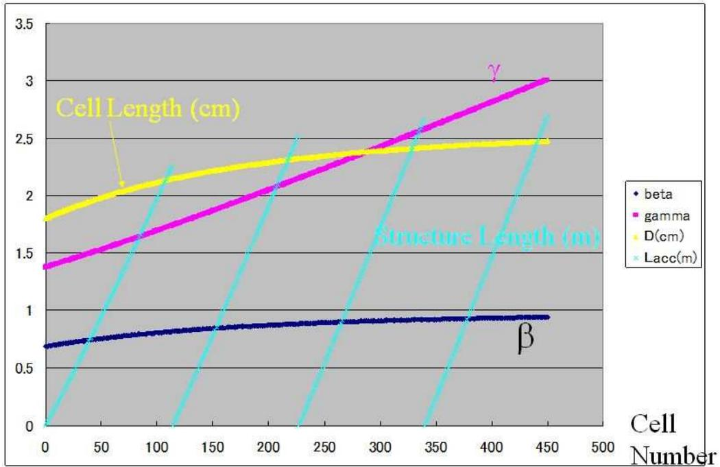
FIG. 32: Cell length corresponding to the muon velocity.
