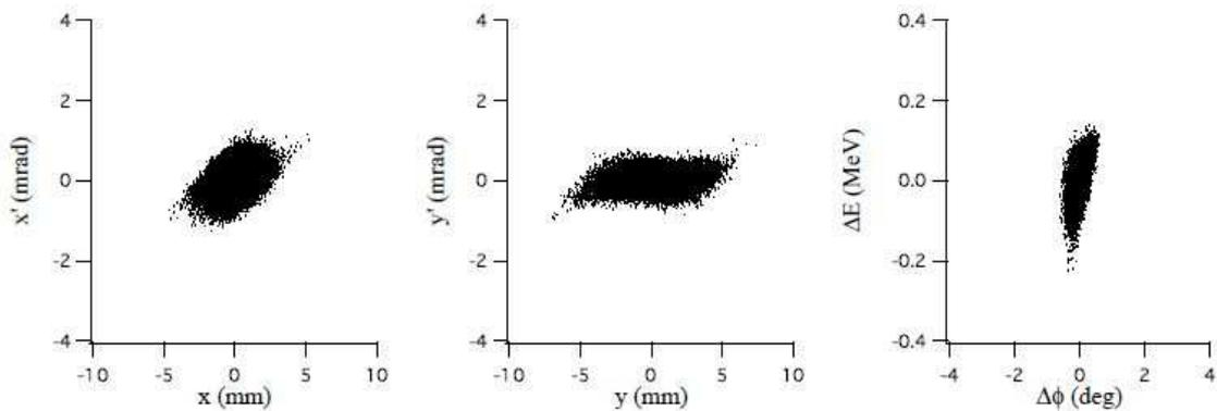
FIG. 30: The particle distribution at the exit of the low- $\beta$  linac simulated with IMPACT
