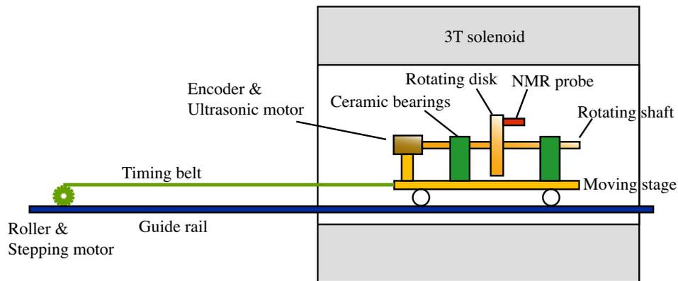
FIG. 50: Overview of the positioning system for the field distribution measurement in the MRI solenoid at NIRS.
