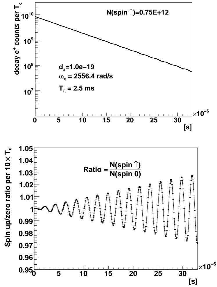
FIG. 69: Top: Time spectrum of positron of  $d_\mu = 10^{-19}$  for  $P_\mu = 1$  (Initial spin direction is parallel to the magnetic field). Bottom: The Ratio of two time spectrum of positron for spin up and spin zero.
