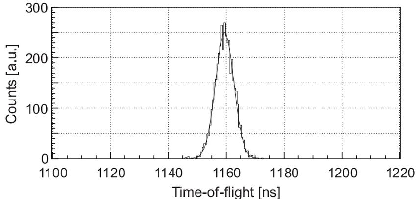
FIG. 21: A time-of-flight spectrum of 9 keV muon beam detected by a MCP at the sample position
