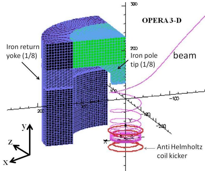
FIG. 44: A kicker system (Anti-Helmholtz coil system) is shown in red lines, in the storage ring magnet. To give an idea of its size, the expected muon beam trajectory, iron pole tip and return yoke are also shown.(Solenoid coil is not shown.)
