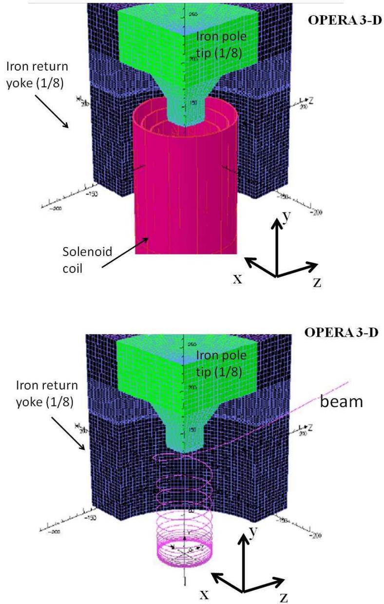
FIG. 38: Top: A conceptual illustration of the storage ring magnet: solenoid coils, one-eighth of iron pole tip and return yoke. Bottom: Calculated spiral trajectory of a single muon particle with  $\gamma_\mu = 3$  by OPERA.
