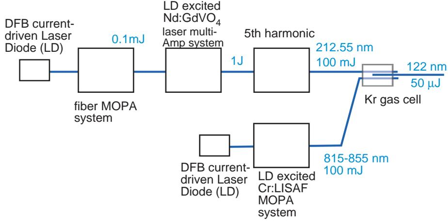
Fig. 1. Conceptual design diagram for new laser system
