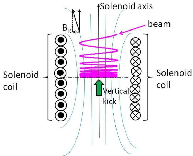
FIG. 37: Schematic representation of spiral injection for our case. A radial fringe field, shown as  $B_R$ , deflects the vertical component of the beam momentum to the horizontal component.
