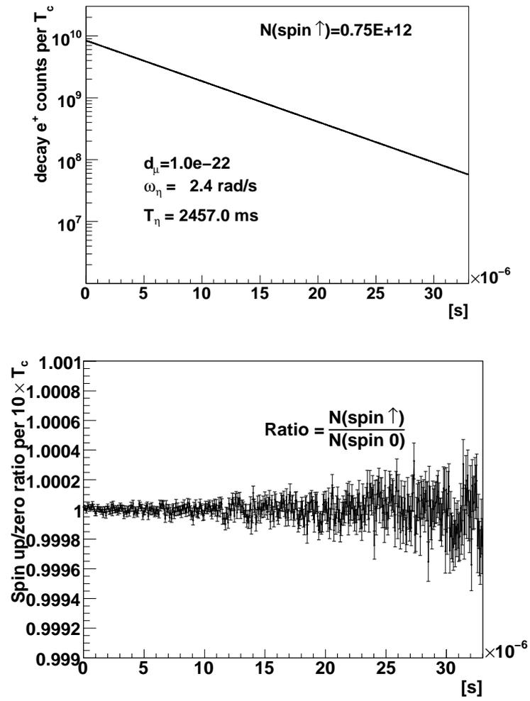
FIG. 70: Top: Time spectrum of positron of  $d_\mu = 10^{-22}$  for  $P_\mu = 1$  (Initial spin direction is parallel to the magnetic field). Bottom: The Ratio of two time spectrum of positron for spin up and spin zero.
