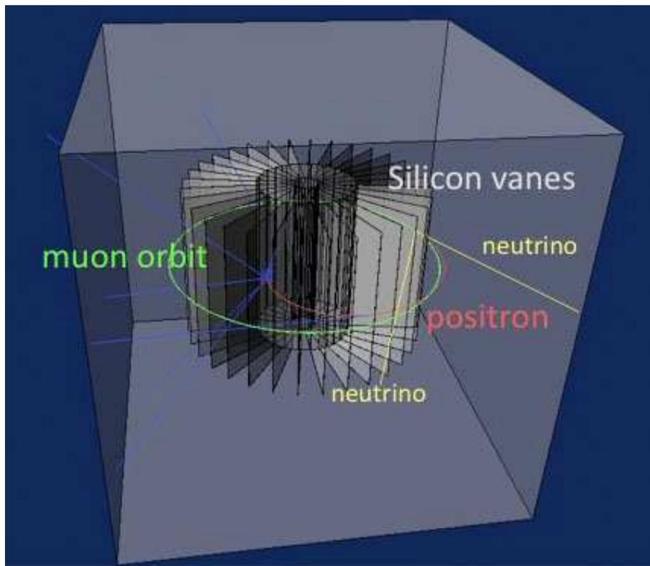
FIG. 66: Layout of the positronium detector system
