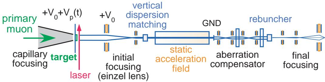
FIG. 27: Schematic setup for the initial acceleration.
