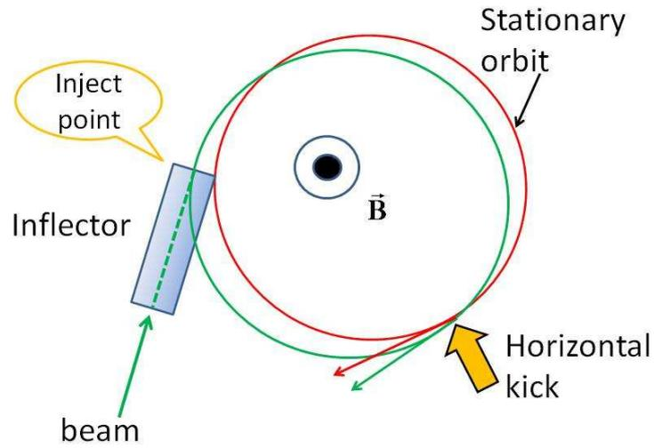
FIG. 36: Injection scheme for previous experiment (BNL  $g-2$ ) from top view. They have inflector and horizontal kicker system.
